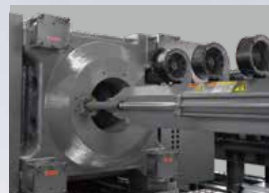
Air fan cooling equipment on the barrel, PID temperature control system.
