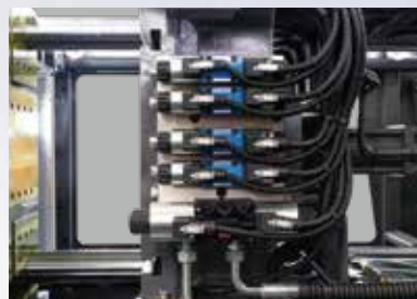
Standard with double core pulling device for Fitting molds.
