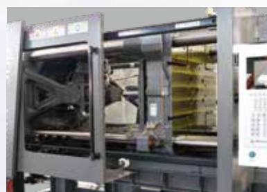
Widened security doors to compatible with core pulling cylinder structure of FITTING MOULD.
