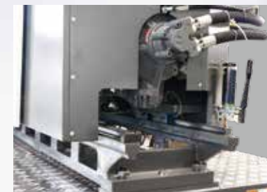
Enlarged charging system with stronger torque of motor to improve plasticization for PVC/CPVC.
